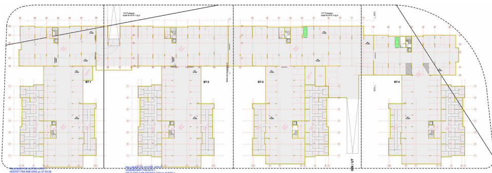
Figure 1. Floor plan of the garages for cases a, b and c (see Table 1). Permission from the architects has been granted.
