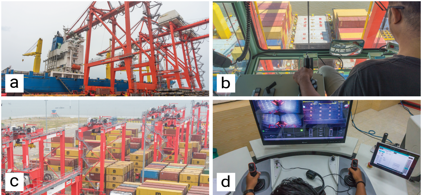
Figure 1: The cranes employed at the container terminal. (a) The STS cranes used for loading and unloading containers to and from containers ships. (b) The cabin used by the operator to control the STS crane. (c) The ARTG cranes used for moving containers between storage yards and transport vehicles. (d) The remote control station used by the operator to control any of the ARTG cranes within the container terminal.
