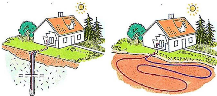
Figure 2.1 Closed loop ground source heat pump (GSHP) technologies: vertical boreholes ( left ) and horizontal collector pipes ( right ). Illustrations by Norman Energiteknikk AS, modified in Gjengedal (2021).
