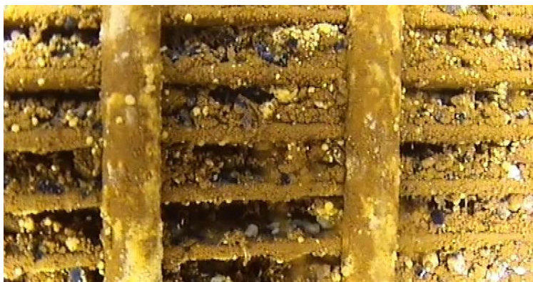
Figure 5.4 Camera inspection from bottom (32.7 m below well top) of Lena terrasse GWHP’s injection well screen (23.5-33.5 m below well top).
