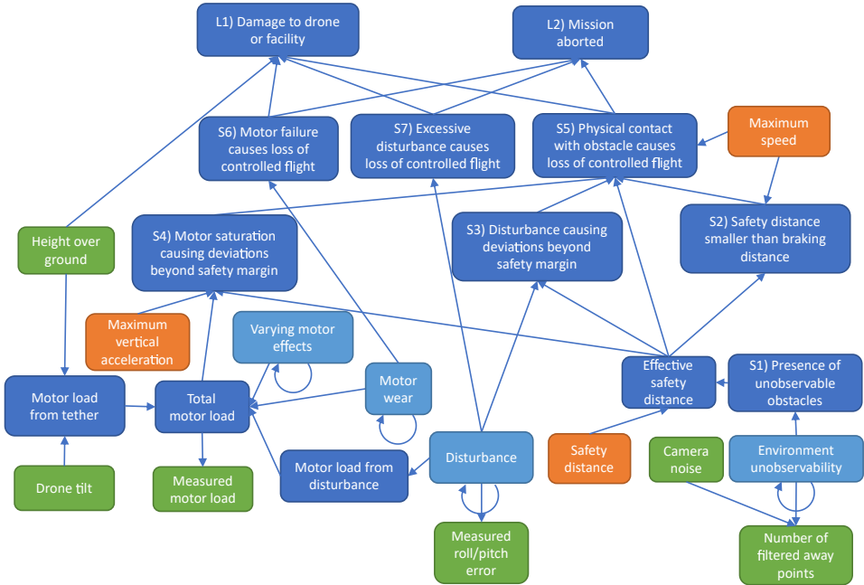
Figure 5.7: DDN for the industrial inspection drone. Dark blue nodes represent intermediate, scenario, and loss nodes. Parameters the supervisory risk controller can control are shown in orange, measurement nodes in green, and underlying causal factors in light blue. The causal factors are dynamic. [L1] and [L2] represent losses introduced in Section 5.3.1 step A1. [S1] to [S7] represents scenarios introduced in Section 5.3.1 step A4
