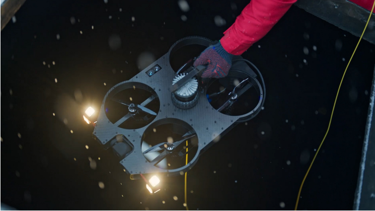
Figure 5.1: The ScoutDI tethered drone used as the case study. Courtesy ScoutDI.
