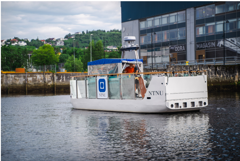
Figure 7.2: The Milliamper 2 ferry used as the autonomous ship in the experiments. Courtesy of Mikael Sættereid.
