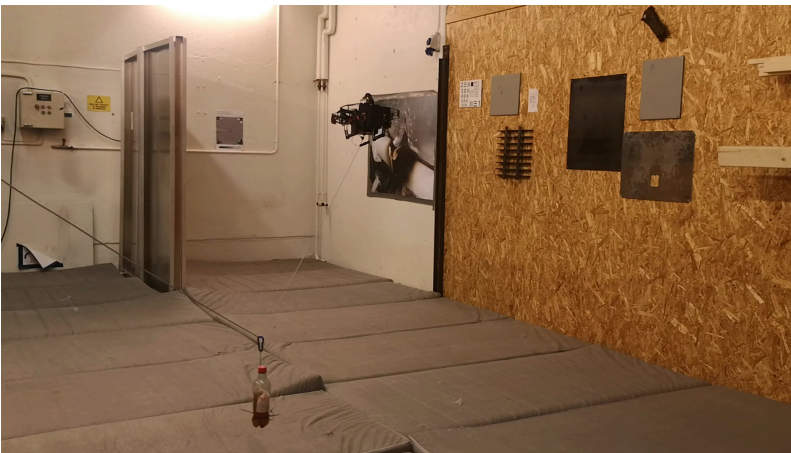
Figure 5.19: The ScoutDI drone flying with a water bottle fastened to an elevated tether. Relevant for Case 7.
