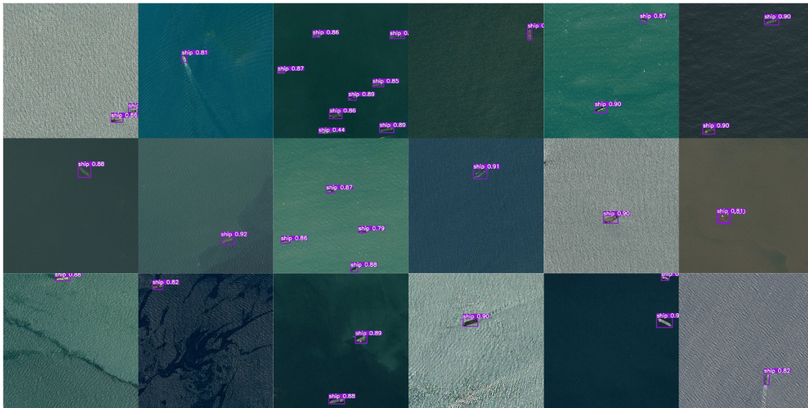
Fig. 8. Test results of the ShipDetectionNet in the scenario of small ships.
