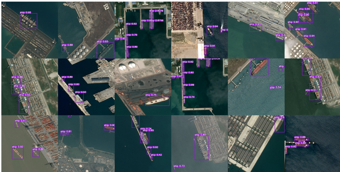
Fig. 7. Test results of the ShipDetectionNet in the scenario of nearshore.
