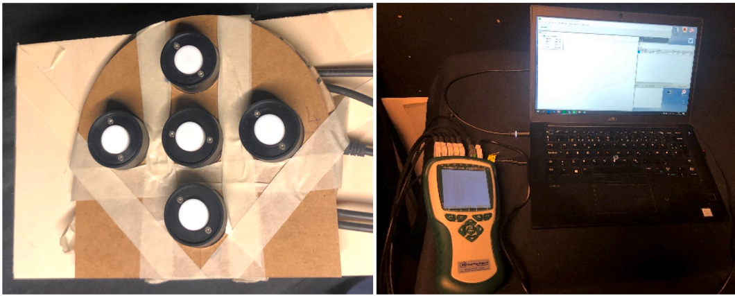
Fig. C3. (left) Measurement instrument Almemo Ahlborn, with photosensors fixed on a circular plate and placed at the tube's exit; (right) logging of measuring data via Ahlborn Almemo logger and Almemo control 6.0 software.
