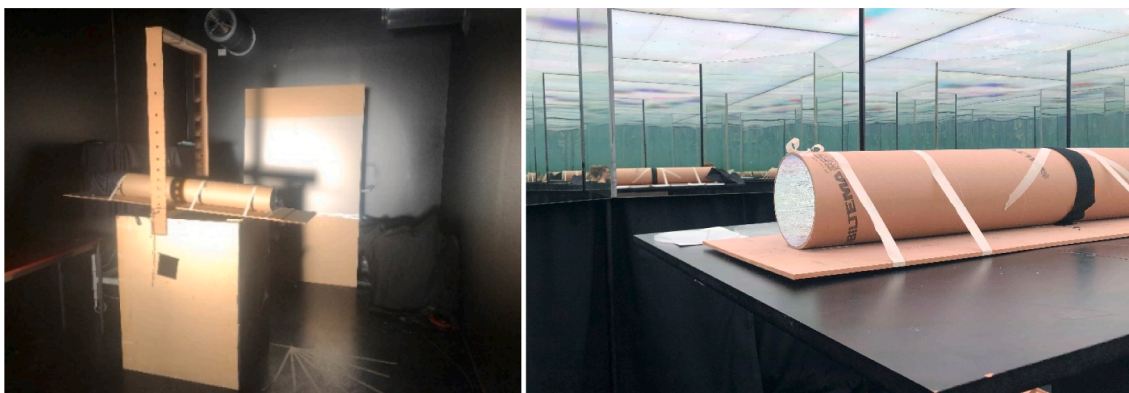
Fig. C2. Model setup in the laboratory study with direct light (left) and diffuse light (right).
