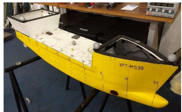
Figure 6: PSV Scale Model Used in the Experiment (Ilanagui 2019)
