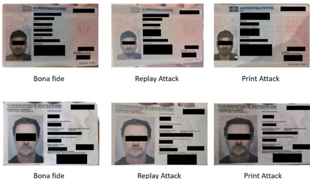
FIGURE 1 An illustration of Bona fide, Replay attack and Print Attack for ID cards. Bona fide images are clear and well defined with no moiré patterns. Replay attack images have different contrast, and images are blurry. The print images have different saturation due to the printer's quality. *Note - Personal information redacted to protect the privacy of the subjects in ID card
