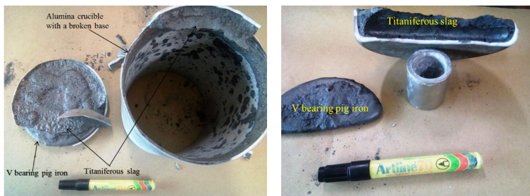
Figure 4: Photograph showing the appearance of the bulk smelting products in alumina crucible
