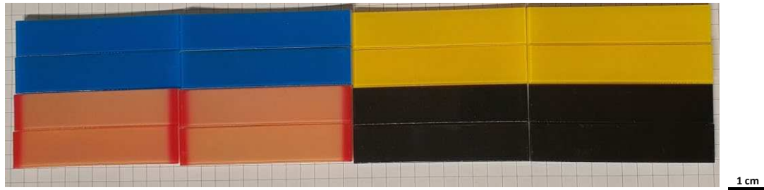
Figure 4. DMA specimens after two weeks of weathering exposure.
