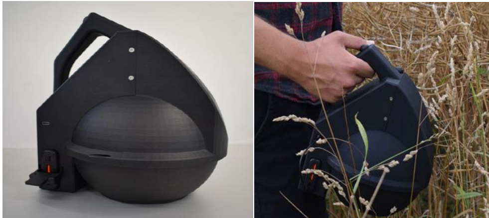
Figure 1. VideometerLite, portable handheld multispectral imaging device.
