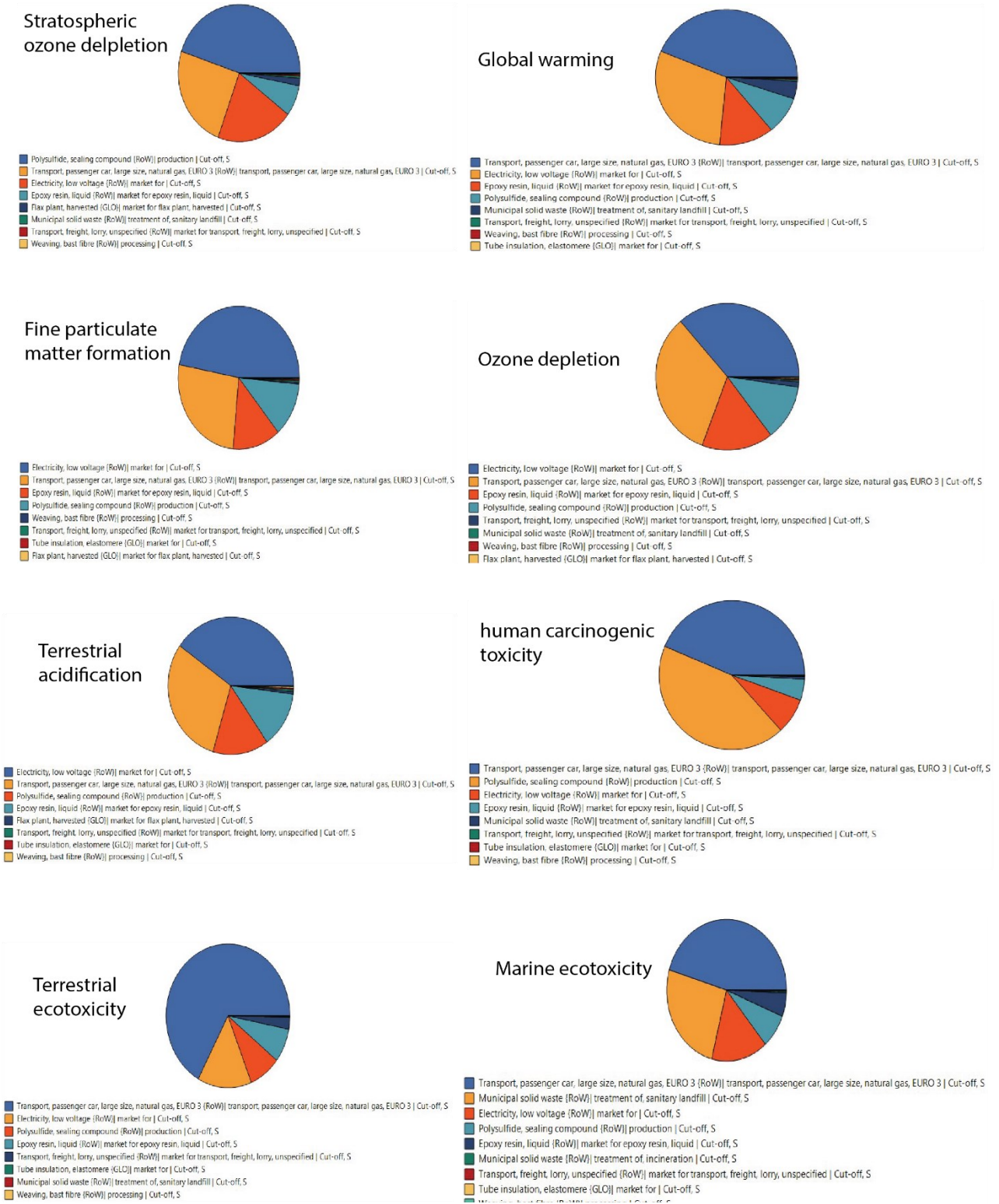
Figure 4.28 Characterization analysis of individual impact indicators for 1.38kg flax fiber composite frame
