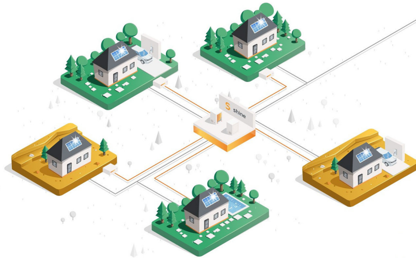
Figure 1: A small LEC with solar production and car batteries as ESS, from (1)
