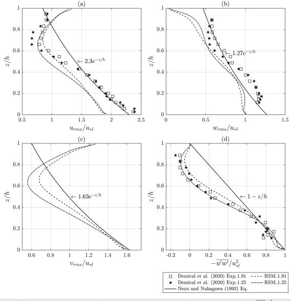
FIG. 17. Comparison of the turbulence profiles at the channel center y/h = 0 (a)  $u_{rms}/u_{\gamma_h}$  (b)  $w_{rms}/u_{\gamma_h}$  (c)  $v_{rms}/u_{\gamma_h}$  and (d)  $-\overline{u'w'}/u_{*i}^2$
