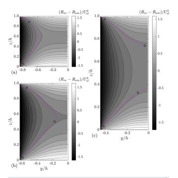
**FIG. 15.** Contour plots of the normalized turbulence anisotropy  $(R_{vv} - R_{ww})/U_{*i}^2$  for the cases (a) RSM\_1.91, (b) RSM\_1.25, and (c) RSM\_0.9.
