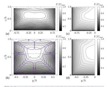
**FIG. 6.** Contour plots of the normalized longitudinal velocities *U/U<sub>max</sub>* for the cases (a) Exp\_1.91 (Demiral *et al.*, 2020), (b) Exp\_1.25 (Demiral *et al.*, 2020), (c) RSM\_1.91, and (d) RSM\_1.25.
