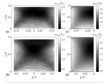
**FIG. 13.** Contour plots of the normalized longitudinal turbulence intensities  $u_{rms}/U_{1}$  for the cases (a) Exp\_1.91 (Demiral *et al.*, 2020), (b) Exp\_1.25 (Demiral *et al.*, 2020), (c) RSM\_1.91, and (d) RSM\_1.25.
