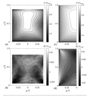
**FIG. 8.** Contour plots of the normalized velocities for the cases with  $a_r = 0.9$  (a)  $U/U_{max}$ —Exp (Demiral *et al.*, 2020), (b)  $W/U_{max}$ —Exp (Demiral *et al.*, 2020), (c)  $U/U_{max}$ —RSM, and (d)  $W/U_{max}$ —RSM.
