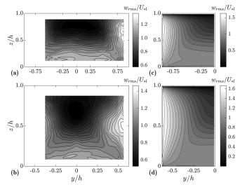
**FIG. 14.** Contour plots of the normalized vertical turbulence intensities  $w_{rms}/U_{1}$  for the cases (a) Exp\_1.91 (Demiral *et al.*, 2020), (b) Exp\_1.25 (Demiral *et al.*, 2020), (c) RSM\_1.91, and (d) RSM\_1.25.
