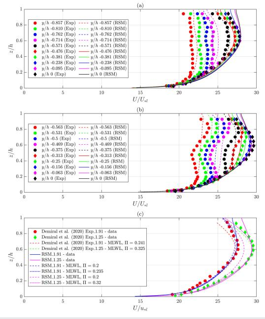
**FIG. 5.** Comparison among the normalized longitudinal velocity profiles obtained from experiments (Demiral *et al.*, 2020) and RSM at (a) different lateral locations for  $a_r = 1.91$ , (b) different lateral locations for  $a_r = 1.25$ , and (c) the channel center y/h = 0 for the obtained data and for the profiles obtained using the modified log-wake-law (MLWL).
