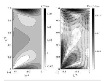
**FIG. 10.** Contour plots of the normalized simulated velocities for the case RSM\_0.9 (a)  $V/U_{max}$  and (b)  $U_{WV}/U_{max}$  with secondary velocity vector plot.
