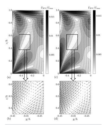
FIG. 12. Simulated secondary velocity vector plots (a) case RSM\_1.1, (b) development of the intermediate vortex for RSM\_1.1, (c) case RSM\_1.05, and (d) development of the intermediate vortex for RSM\_1.05.
