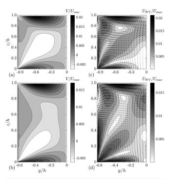
**FIG. 9.** Contour plots of the simulated (a) normalized lateral velocity  $V/U_{max}$  for the case RSM\_1.91, (b)  $V/U_{max}$  for the case RSM\_1.25, (c) normalized resultant secondary velocity  $U_{WV}/U_{max}$  with vector plot for the case RSM\_1.91, and (d)  $U_{WV}/U_{max}$  with vector plot for the case RSM\_1.25.
