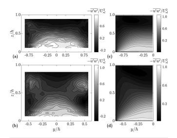
**FIG. 16.** Contour plots of the normalized primary specific Reynolds shear stress  $-\overline{u'w'}/U_{*l}^2$  for the cases (a) Exp\_1.91 (Demiral *et al.*, 2020), (b) Exp\_1.25 (Demiral *et al.*, 2020), (c) RSM\_1.91, and (d) RSM\_1.25.
