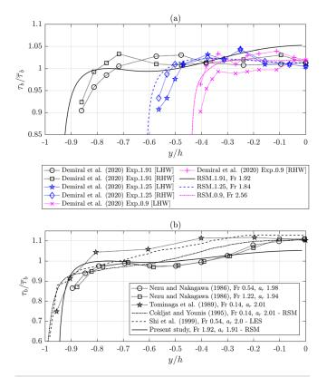
**FIG. 18.** Comparison of the normalized bed shear stress distributions (a) between Exp (Demiral *et al.*, 2020) and RSM cases and (b) among several cases with  $a_r$  around 2.0 (LHW = left half width, RHW = right half width).
