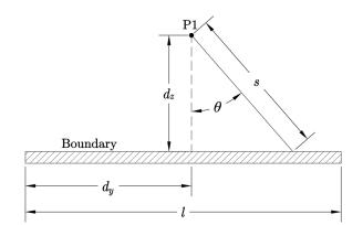
FIG. 2. Notations for the calculation of average distance of point P1 from a boundary [after Cokijat (1993); Naot and Rodi (1982)].
