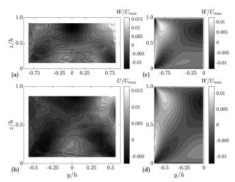
FIG. 7. Contour plots of the normalized vertical velocities *W/U<sub>max</sub>* for the cases (a) Exp\_1.91 (Demiral *et al.*, 2020), (b) Exp\_1.25 (Demiral *et al.*, 2020), (c) RSM\_1.91, and (d) RSM\_1.25.
