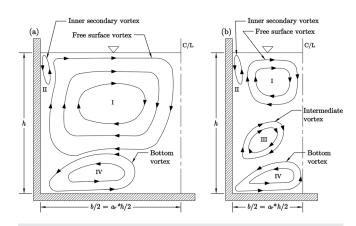
**FIG. 1.** Secondary currents in left half of straight fully developed open channel flows for (a) narrow channel with  $a_r$  around 2 [after Kang and Choi (2006)] and (b) very narrow channel with  $a_r$  around 1 [based on Broglia *et al.* (2003); Naot and Rodi (1982) and the present study].
