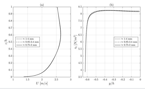
FIG. 4. Grid convergence results for the case RSM\_1.25 (h = 0.16 m and Fr = 1.84), which compare the (a) longitudinal velocity profiles at the channel center and (b) lateral variation in the bed shear stress.
