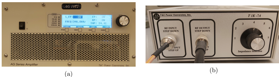
Figure 3.2: Experimental equipment; signal generator AG1012 (a), and impedance matching unit (b).
