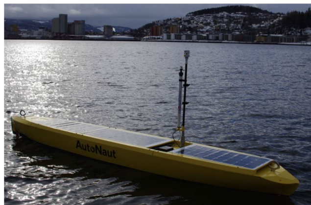
FIGURE 3. The NTNU Autonaut [20] is propelled by the motion of the waves. The vehicle's length is 4.6 m and the mass is 250 kg.
