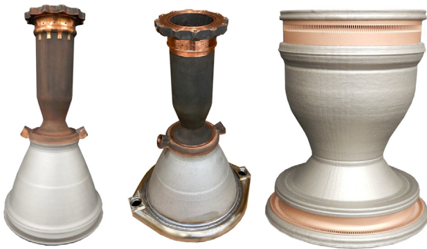
Fig. 20. a: Bimetallic 7k Coupled Chamber using L-PBF GRCo-42 with HR-1 DED Integrated Nozzle (b: complete with manifolds). c: Bimetallic 40k Chamber built using L-PBF GRCo-42 liner and HR-1 DED Jacket. (Courtesy: NASA)[209].
