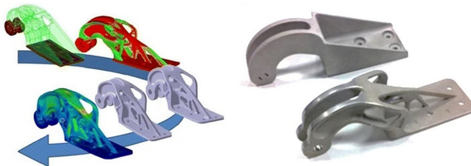
Fig. 2. TO and AM of Airbus A320 nacelle hinge bracket. Left: TO design process. Right: Original bracket (top) and final TO optimized design (bottom) [116,117]. Original steel bracket = 918 g; TO and AM bracket in Ti6Al4V = 326 g. Copyright: Airbus.
