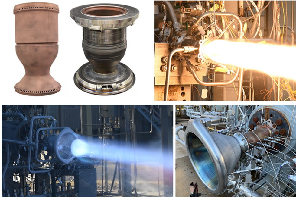
Fig. 5. Examples of fully AM thrust chamber assemblies hot-fire tested at NASA MSFC including injectors, combustion chambers, and channel-cooled nozzles, including L-PBF GRCo-84, L-PBF GRCo-42, bimetallic L-PBF and DED, and LP-DED NASA HR-1. (Courtesy: NASA) [135–137]
