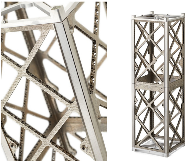
Fig. 10. nTopology and AFIT lattice CubeSat bus structure. Credit: nTopology [155].
