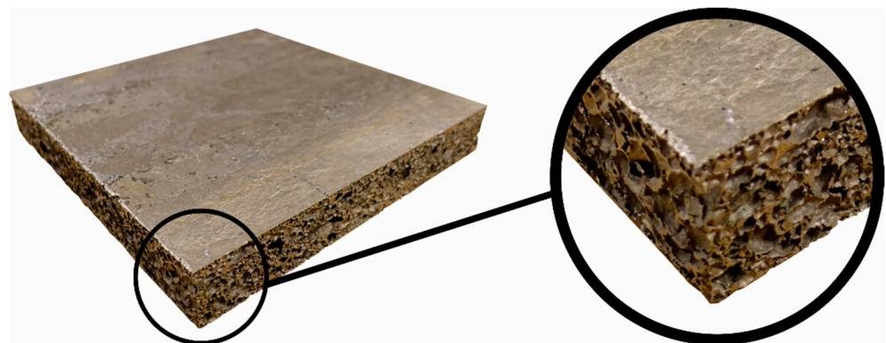
Figure 1. Typical aluminium foam panel applied in the ballistic impact tests, showing the external skins and the inhomogeneous porous core.
