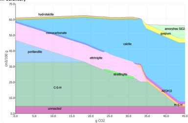
Figure 10. Thermodynamic modelling of the equilibrium phase assemblage during carbonation of a white PC at W/B = 0.5, 20°C and degree of hydration 90%: A) with CemGEMS and B) using GEM-Selektor (adapted from [75]). In both diagrams, the undegraded cement paste is shown on the left-hand side, while moving to the right, more and more CO<sub>2</sub> (mass in grams) reacts with the hydrates.
