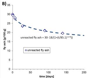
Figure 4. A) measured (symbols) and modelled (mP&K model: solid lines; 4PL fit: dashed line) clinker reaction in PC as a function of time: equations and parameters see Supplementary Material B; B) measured (symbols) and modelled (lines) fly ash reaction in a blend containing PC, fly ash and limestone using the 4PL fit based on experimental data reported in [30].
