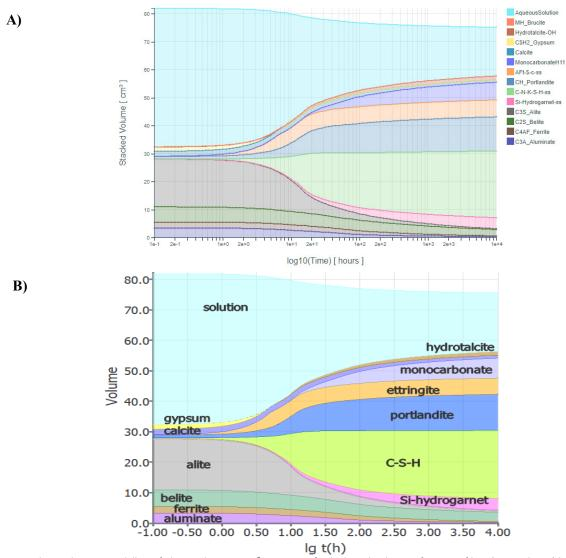
Figure 5. Thermodynamic modelling of phase volumes in cm<sup>3</sup> per 100 g of anhydrous binder as a function of log<sub>10</sub>(time in hours) based on the cement composition and mP&K parameter given by De Weerdt et al. [30] using a) CemGEMS and b) GEM-Selektor at a water/solid ratio w/b = 0.5 and a temperature of 20°C (screen images).
