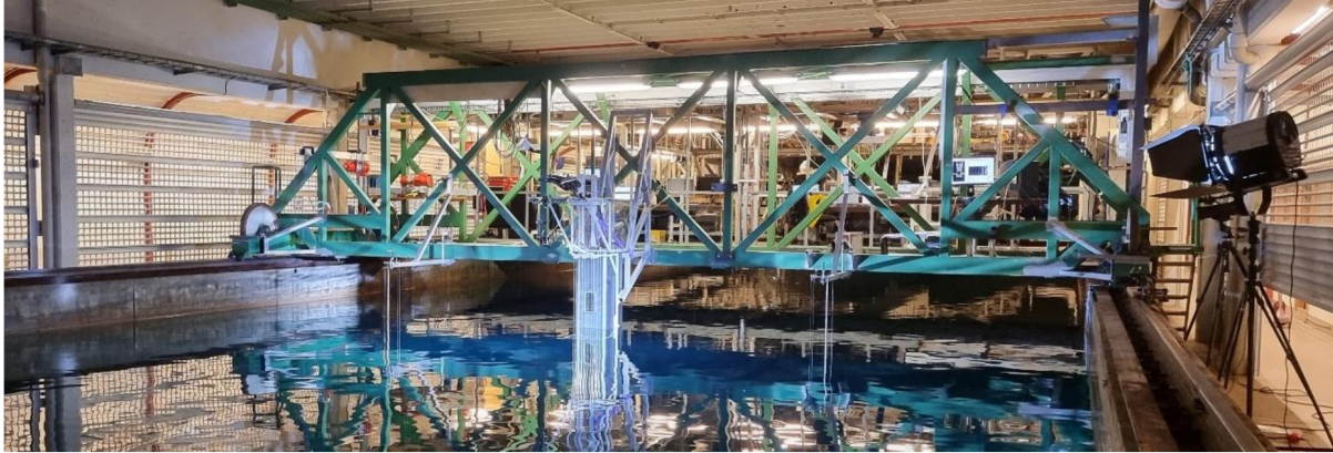
Figure 1: Experimental setup: the rectangular cylinder with flexible panel installed against the wave-maker. The structure is mounted on the carriage bridge.
