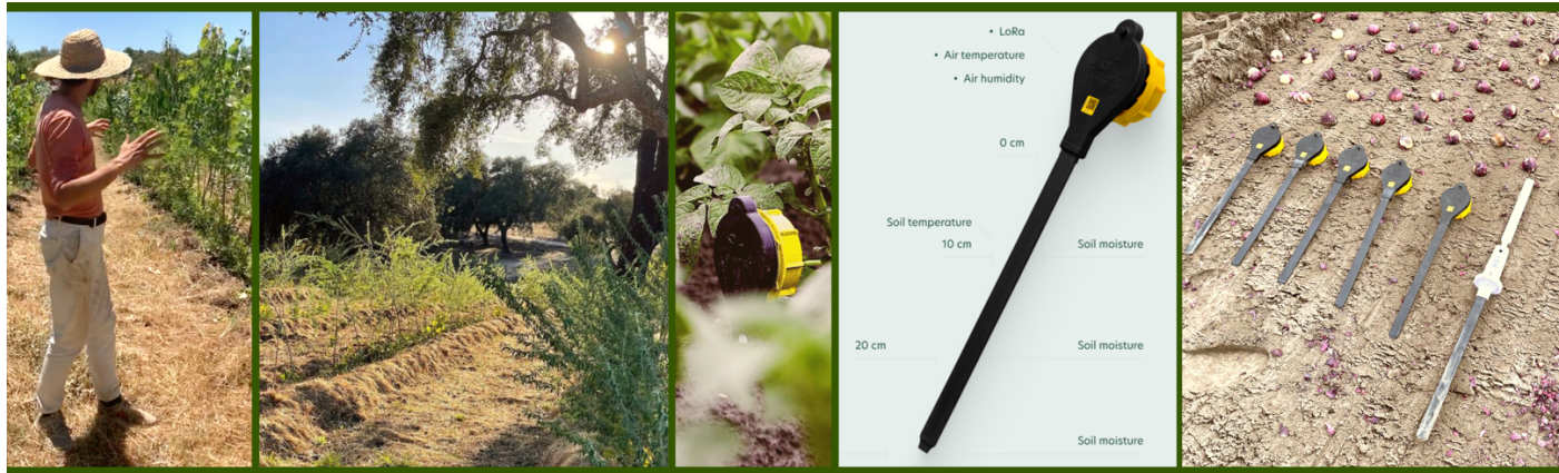
Figure 14: August 2022. Fieldwork on-site Quinta das Abelhas, Alentejo region of Portugal. Farm21 intelligent sensors for measuring top and below the ground.
