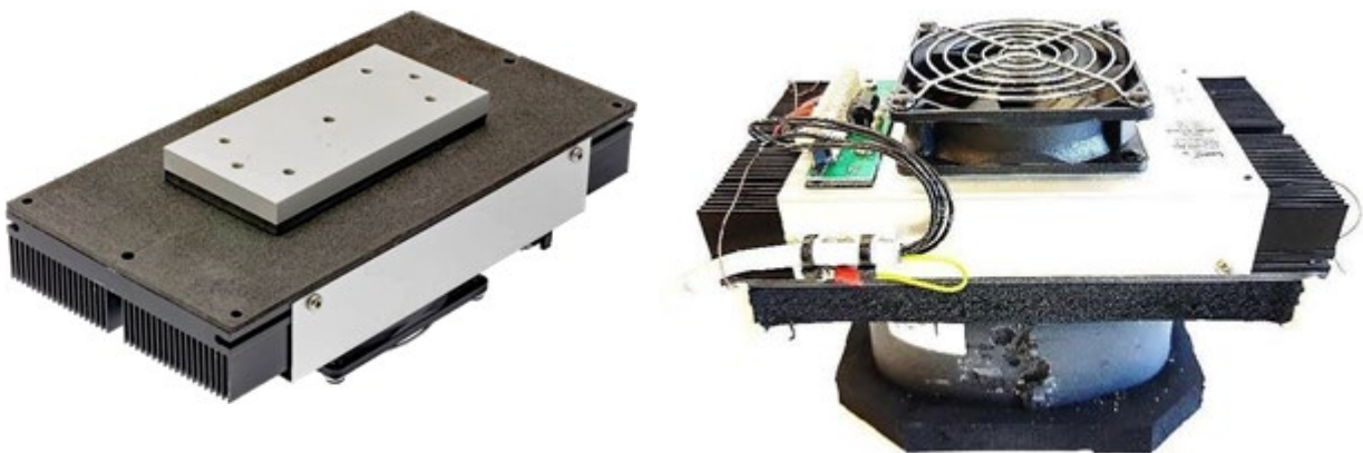
Figure 6 – Experimental set-up. Left: Peltier element mounted on cooling fins with fan (upside down). Right: Temperature control unit mounted on mortar specimen.
