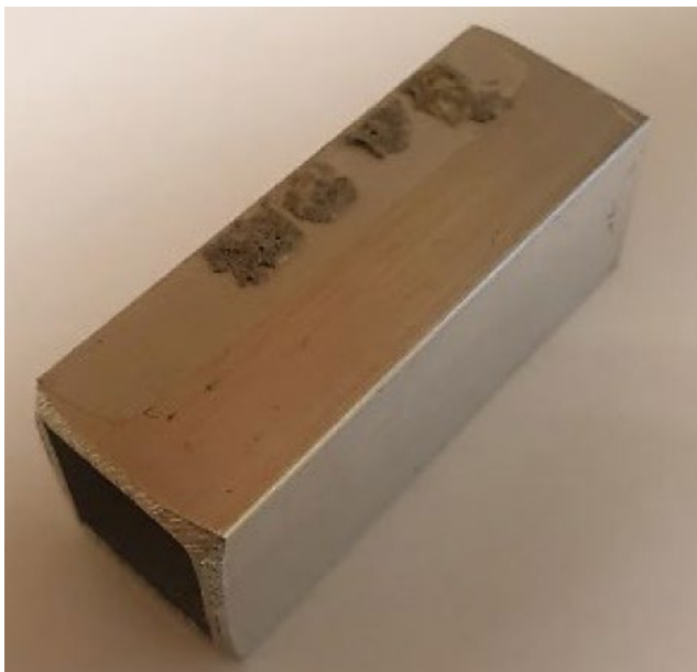
Figure 9 –Top: Scaled material after sieving. Bottom, left: Flakes mounted on a hollow steel bar with quadratic cross section by double-sided tape. Bottom, right: Digital photos taken perpendicular and parallel to the surface of the steel bar made it possible to determine thickness ( T ), length ( L ) and width ( W ) of the individual flakes accurately. (Illustrations from [14]).
