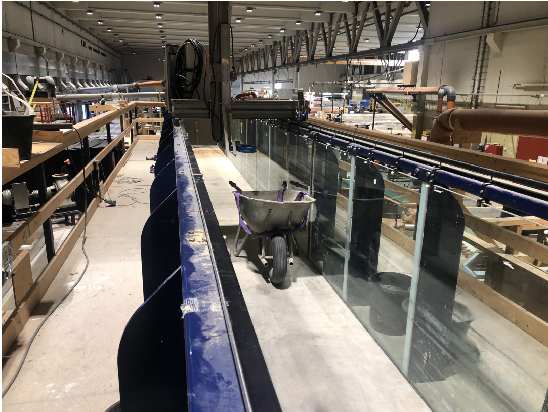
Figure 4.2: The flume where the physical model will be built. The width of the flume is 1 m.
