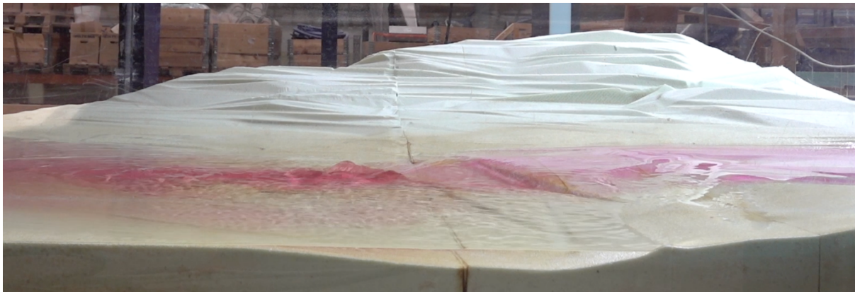
Figure 5.1: Picture of the hydraulic jump induced for Q=140 \text{ m}^3/s , seen from camera 5. Flow direction from right to left.
