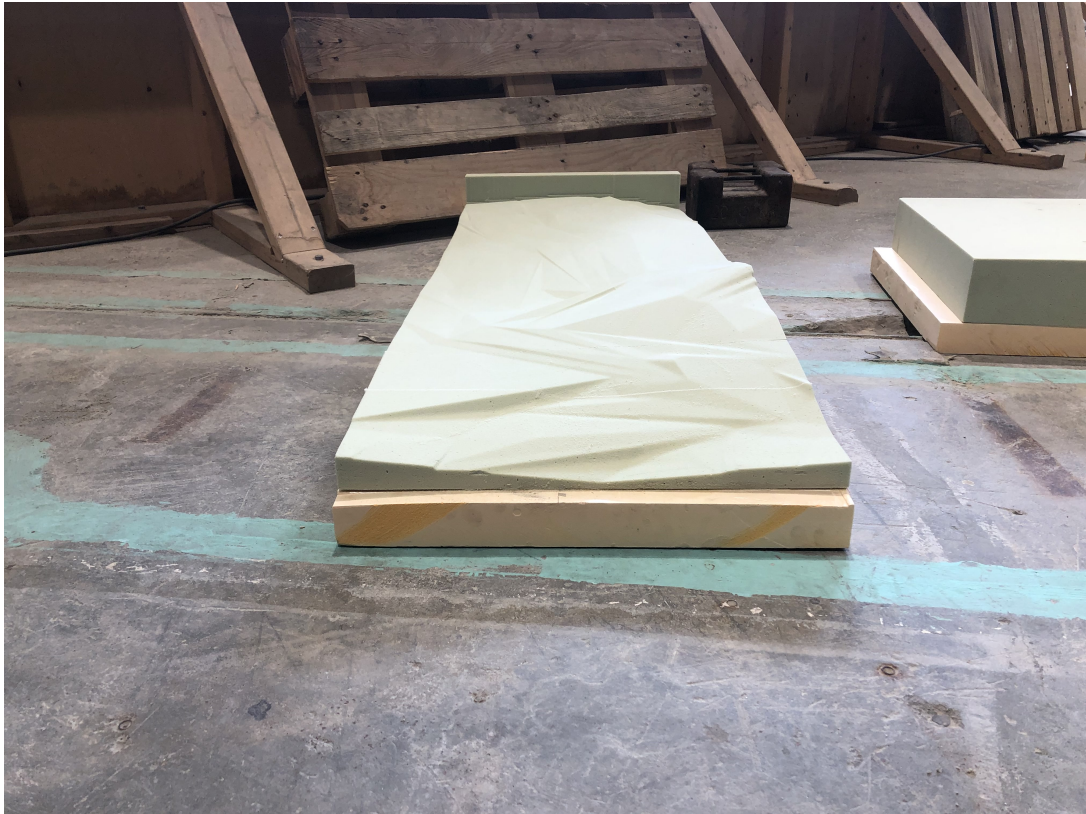
Figure 4.6: The finish result after printing the river bed on polyurethane.
