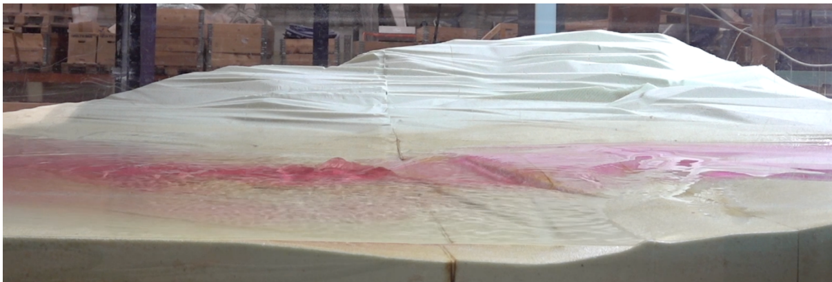
Figure 5.21: Q = 140 \text{ m}^3/\text{s} . Comparison of the highest and lowest water discharge tested in the flume. Flow direction from right to left.
