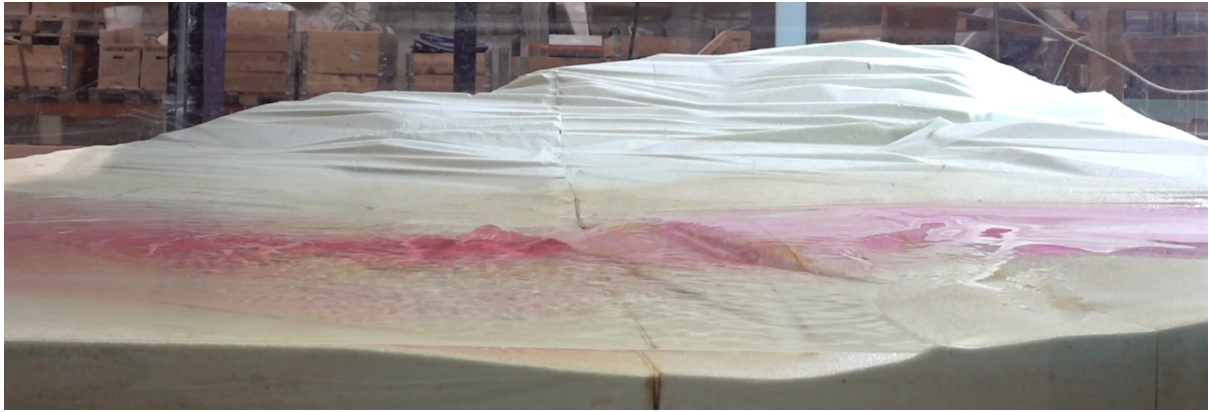
Figure 6.5: Physical model, Q = 140 \text{ m}^3/\text{s} . Flow direction from right to left.
