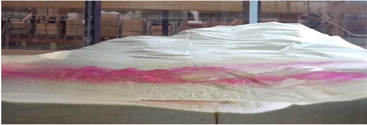
Figure 5.22: Q = 400 \text{ m}^3/s . Comparison of the highest and lowest water discharge tested in the flume. Flow direction from right to left.
