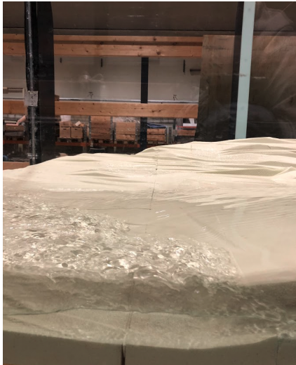
Figure 4.14: The hydraulic jump over the model for a random discharge.
