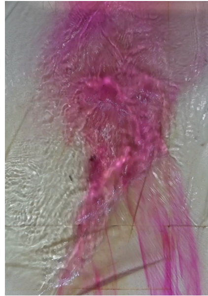
Figure 5.13: Picture of the hydraulic jump for Q = 289 \text{ m}^3/\text{s} in Nidelva, seen from camera 3.
