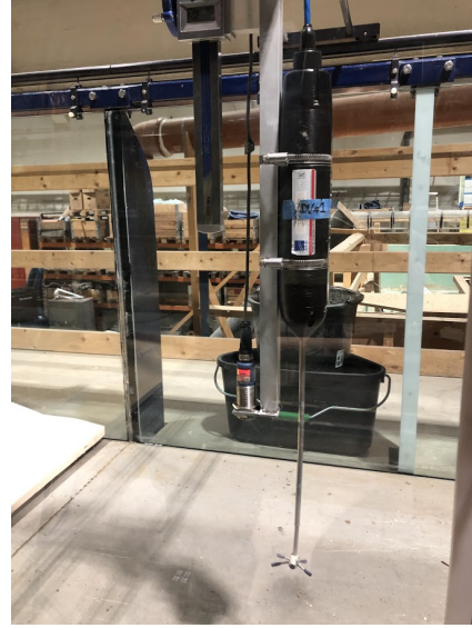
Figure 4.13: The placing of the ADV, Vectrino
