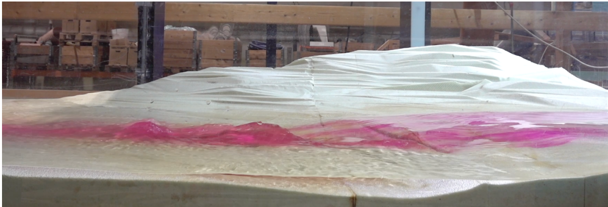
Figure 5.11: Picture of the hydraulic jump induced for Q=289 \text{ m}^3/s , seen from camera 5. Flow direction from right to left.
