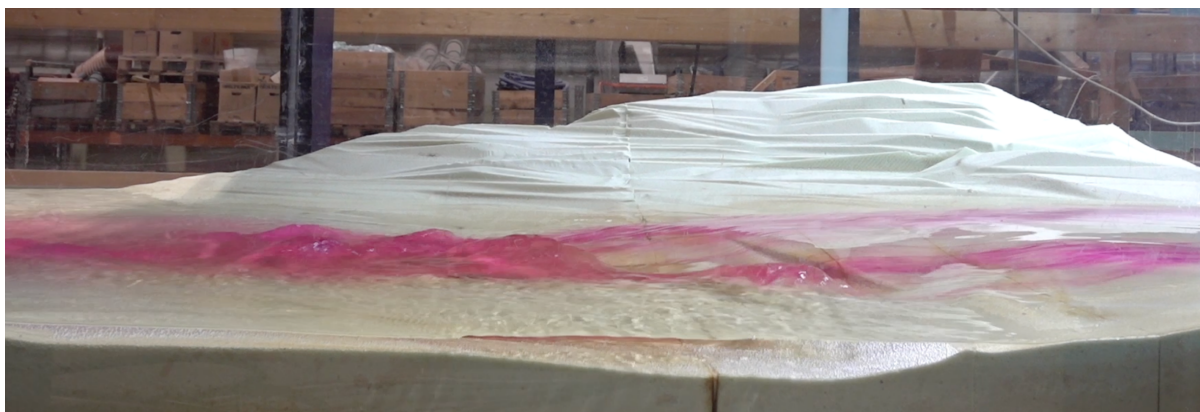
Figure 5.16: Picture of the hydraulic jump induced for Q=400 \text{ m}^3/s , seen from camera 5. Flow direction from right to left.
