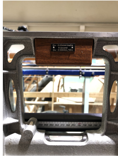
Figure 6.12: The tilting of the flume after adjustment.
