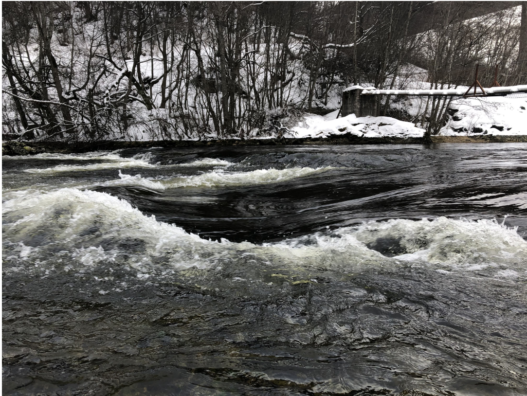
Figure 3.1: A hydraulic jump in the Drop of Death, Nidelva, taken 23. February 2022. Q = 102.4 \text{ m}^3/\text{s}
