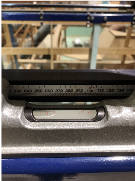
Figure 6.11: The tilting of the flume before adjustments were made.
