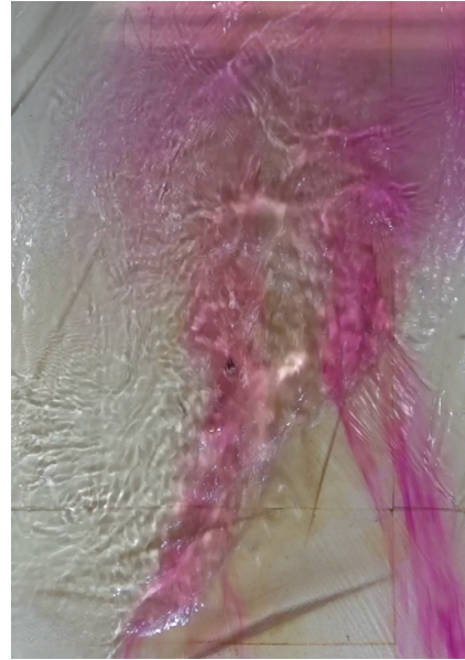
Figure 5.18: Picture of the hydraulic jump for Q = 400 \text{ m}^3/\text{s} in Nidelva, seen from camera 3.
