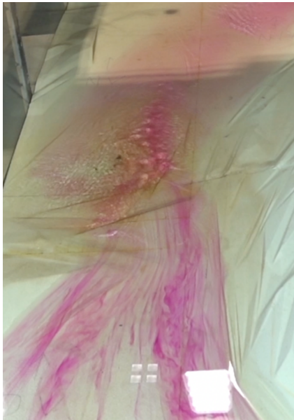
Figure 5.2: The flow situation for Q=140 \text{ m}^3/\text{s} seen from upstream, camera 1.
