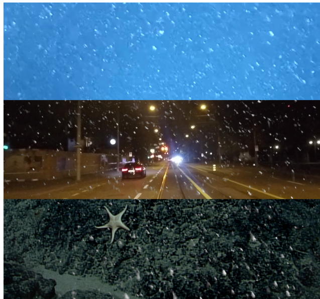
Figure 1. In our approach, we extract marine snow from underwater footage with untextured background (top), and superimpose this snow on arbitrary footage to create labelled training data (bottom images) for training snowflake detectors .
