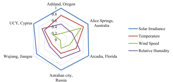
FIGURE 7. Relative importance of weather parameters for various locations based on correlation study with respect to the PV output power [12], [33]–[37].
