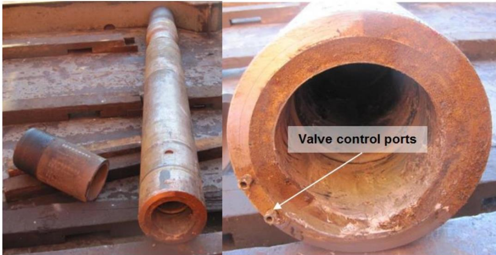
Figure 1.1. Subsurface safety valve assembly (left) and the fracture surface (right) [4].
