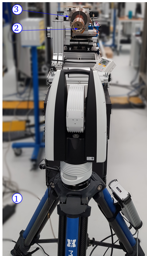
Figure 3.12: Leica AT930 laser tracker setup for the validation measurements of the translating coil fluxmeter measurement system. It shows the laser tracker, (1), the fixed target on the inside of the measurement head, (2), and the target on the external fiducial of the magnet, (3).
