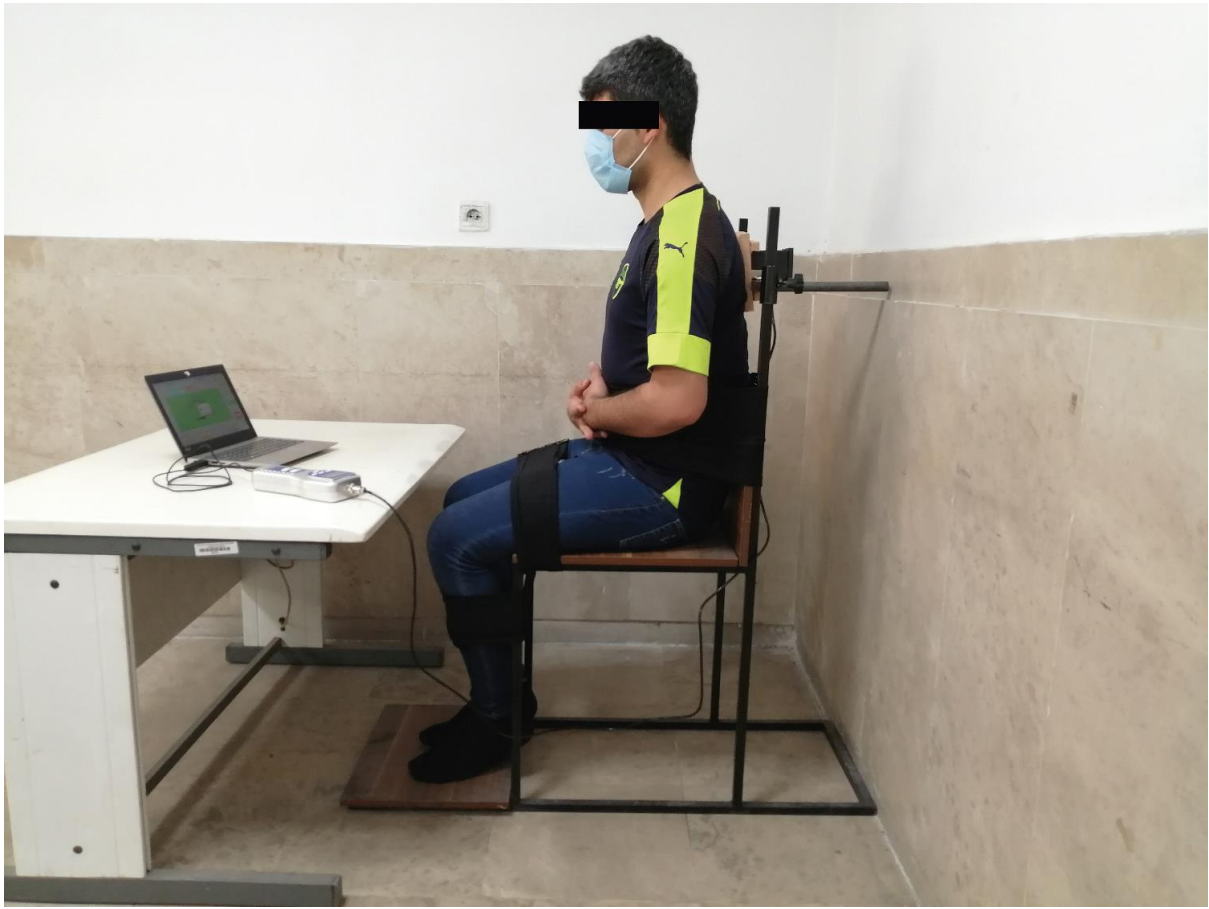
Figure 2. Assessing isometric back extensor strength and endurance using the designed setup.
