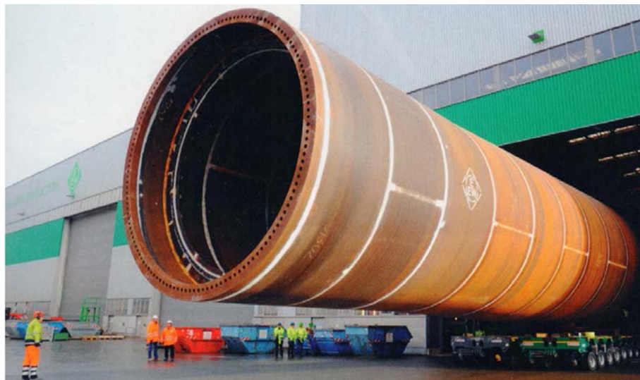
Figure 20. A 1302.5 tonne monopole. Reproduced with permission from [159]. [Source: EEW SPC].
