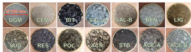
Fig. 5. (Color) RLTT samples: unbound granular material (UGM), cement (CEM), bitumen (BIT), calcium chloride salt (SAL-A), mineral mixture salt (SAL-B), sodium bentonite (BEN), lignosulfonate (LIG), reduced sugar (SUG), petroleum resin (RES), polyurethane (POL), acrylate (ACR), styrene butadiene (STB), and acetate type A (ACE-A) and type B (ACE-B).
