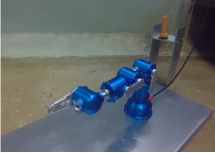
Fig. 5. Experimental setup of manipulator and object out of sight in the pool.
