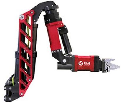
(b) The electric Eca robotics arm 7E, produced by ECA Group [64].
