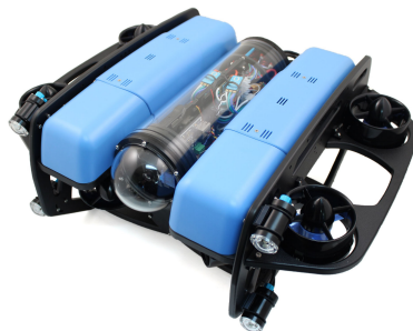
(b) Class II ROV, the BlueROV2, produced by BlueRobotics [8].
