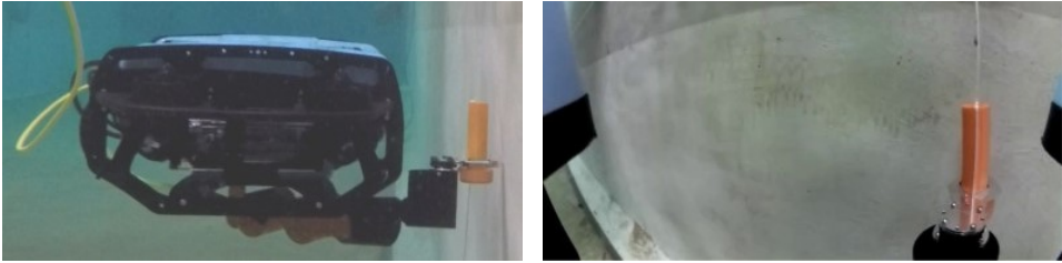
(a) The UVMS successfully grasping the object, seen from outside. (b) The UVMS successfully grasping the object, seen from the vehicle's camera.
