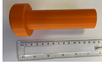
Fig. 4. The cylinder object to be grasped in the experiments. The cylinder is 120mm tall, has an upper diameter of 30mm and a lower diameter of 50mm.
