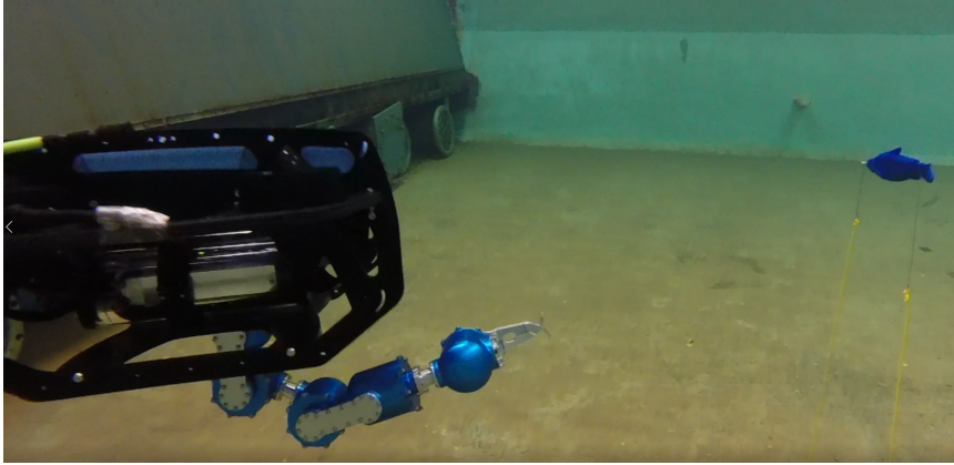
Figure 4.23: UVMS in DP operations in the MC-lab with relevant object in front of the vehicle.
