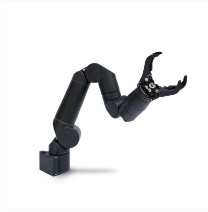
(a) The electric Bravo 7 manipulator, produced by Blueprint Lab [32].
