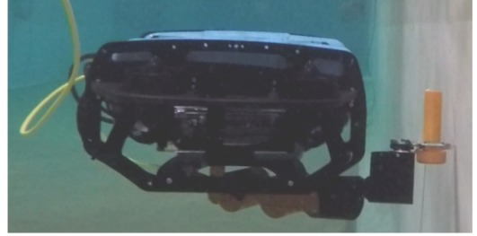
Fig. 14. The UVMS successfully grasping the object seen from the outside during the second grasping operation.
