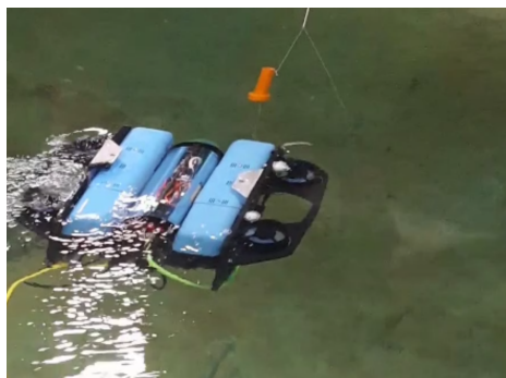
(a) The BlueROV2 performing DP relative to the relevant object in the MC-lab pool.
