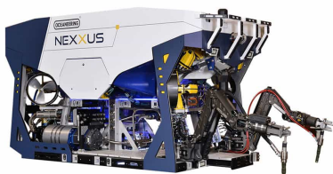
(a) Class III ROV, the NEXXUS ROV, produced by Oceaneering [50].
