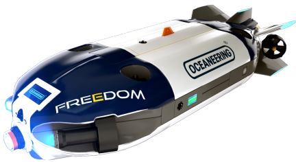
(c) The Freedom resident ROV, produced by Oceaneering [48].
