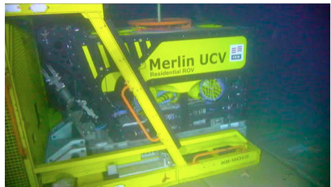
Fig. 2. A Merlin Resident ROV with its “garage” from IKM. Image courtesy of IKM.
