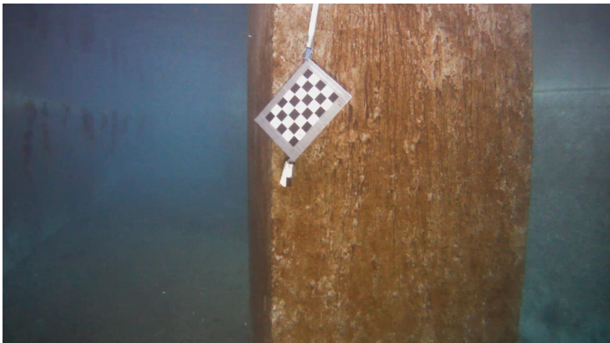
Figure A3.2. Setup for recording the reference video used to calibrate the internal- and external camera parameters for the Blueye ROV in 2021. Here the checkerboard is quite far away and as a result does not cover enough of the screen to be used sufficiently for camera calibration. See figure 2.8 for a closer view of the checkerboard-reference plate. Image: Malin Bø Nevstad, 2021.
