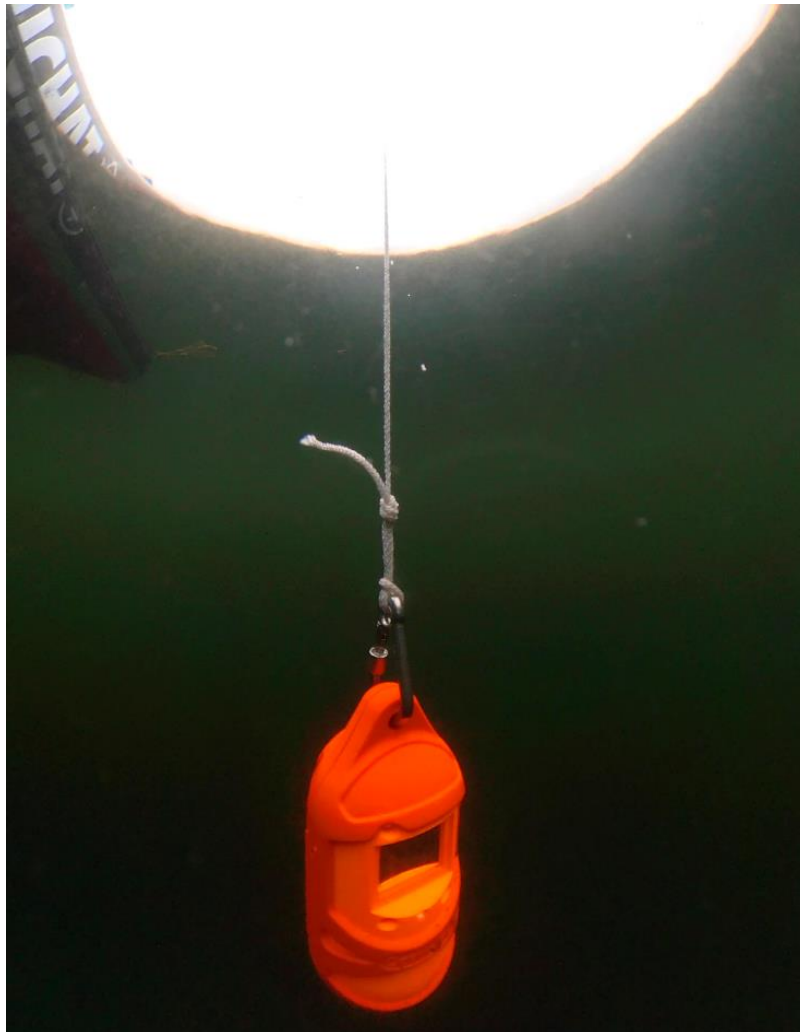
Figure 2.16 360-image of the SonTek CastAway-CTD during vertical profiling of temperature and salinity in Karihavet during fieldwork November 2021. Photo: Geir Johnsen, 2021, with permission.
