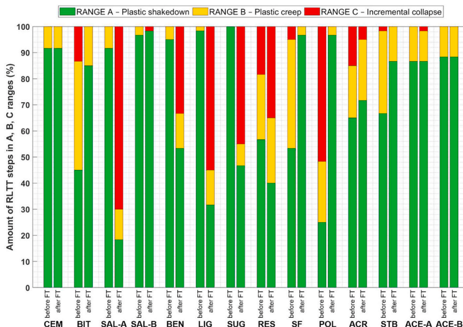
Fig. 11. Classification of each RLTT step based on the permanent deformations measured before and after FT cycles.
