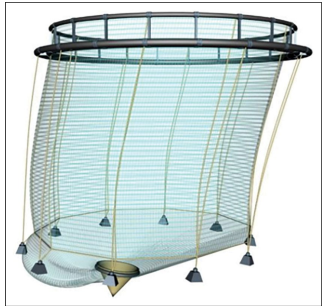
Figure 1. Floating fish farm with circular plastic collar consisting of two tori that are nearly semi-submerged in calm water, the railing, jump net, netting, dead fish removal system, rope framework, and bottom weights (Sintef Fisheries and Aquaculture).
