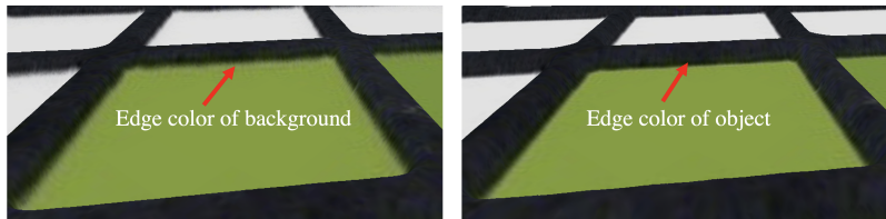
Figure 2.5: Example of edge colors coming from background and object, rendered in Canon Touchstone software at 1 mm elevation and zoomed for illustration purpose. The height map of the image was filtered to reduce effect of black wall and intensity adjusted to reach the intended maximum elevation, and morphological operation was applied to the height map (right side version). The image was used in Article B .
