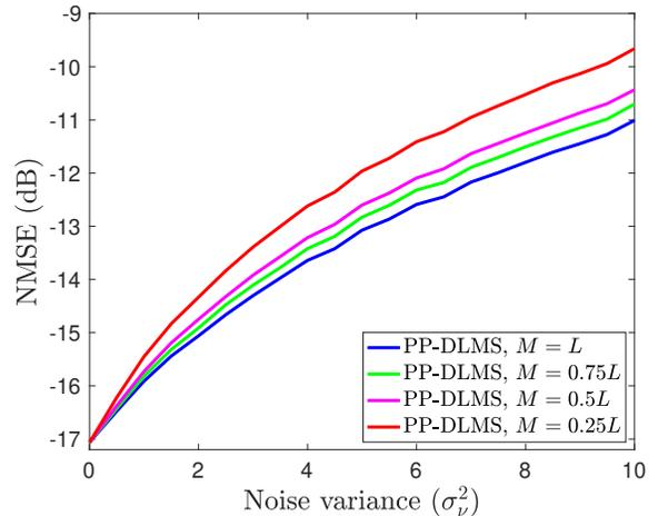
Fig. 2: Network-level MSE (in dB) for different values of  $M$ , i.e., the portion of the shared information, versus injected noise variance  $\sigma_\nu^2$ .
