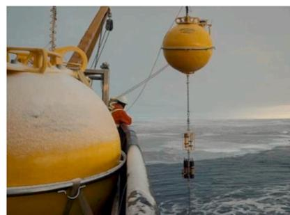
Subsurface mooring buoy redeployment at site location
