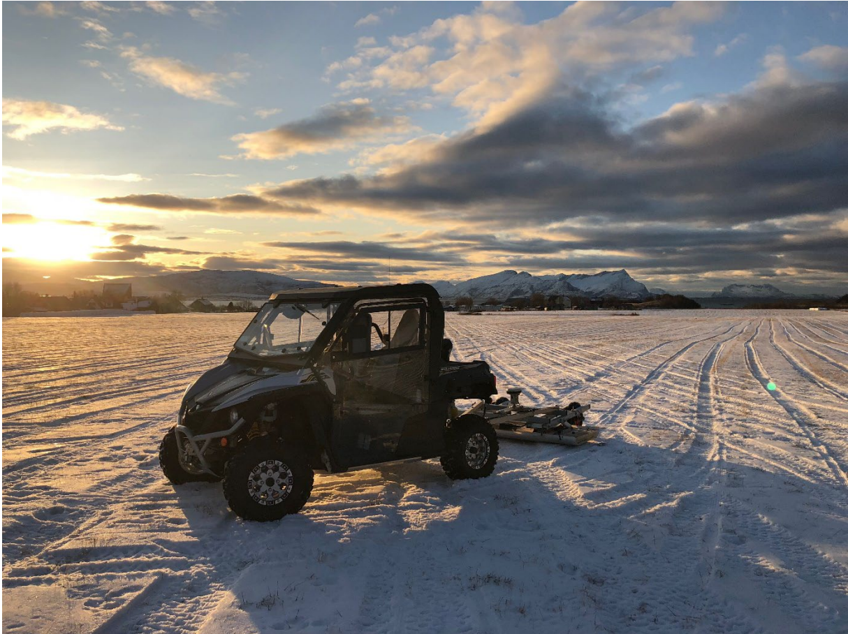
Figure 1: Performing a ground-penetrating radar survey in Northern Norway. Photo: Arne Anderson Stamnes
