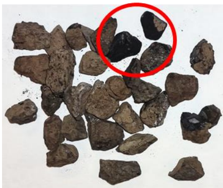
Figure 4-60: Shows the +9.5 mm particles from the Nchwane ore sample reduced in the low pO_2 gas mixture at 605 °C.
