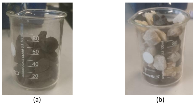
Figure 3-1: (a) 150 g Nchwanging ore and (b) 75 g Comilog ore and 75 g quartz.
