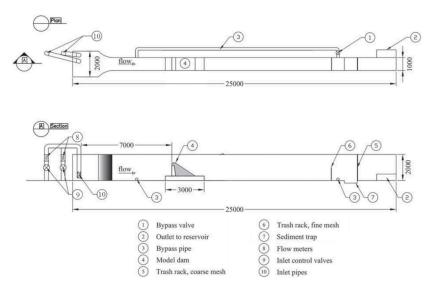
**Figure 3.** Representation of the flume present at the hydraulic laboratory of NTNU (Trondheim) used for the 9 setups introduced in this work. Modified from Kiplesund et al. [22].
