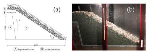
**Figure 6.** (**a**) Depiction of experimental setup of half dam model with core and (**b**) image of dumped riprap model with such setup from [26].
