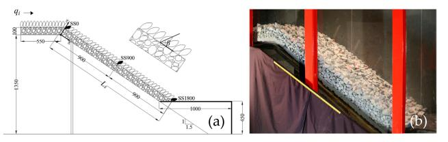
**Figure 5.** From Ravindra et al. [9], (**a**) depiction of experimental set-up of riprap model unsupported at the toe and (**b**) image of dumped riprap model with such setup.
