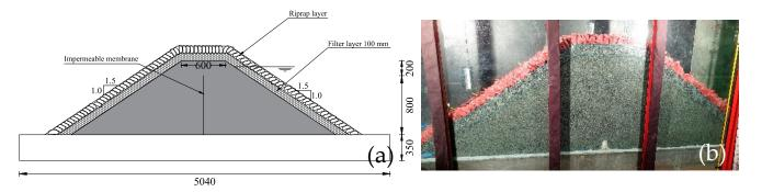
**Figure 8.** (a) Depiction of experimental setup of full dam model with flexible core, and (b) image of placed riprap model with such a setup.
