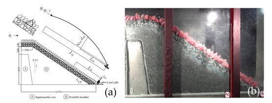
**Figure 7.** (a) Depiction of experimental setup of half dam model with core and placed riprap supported at the toe and (b) image of the model built in the flume.
