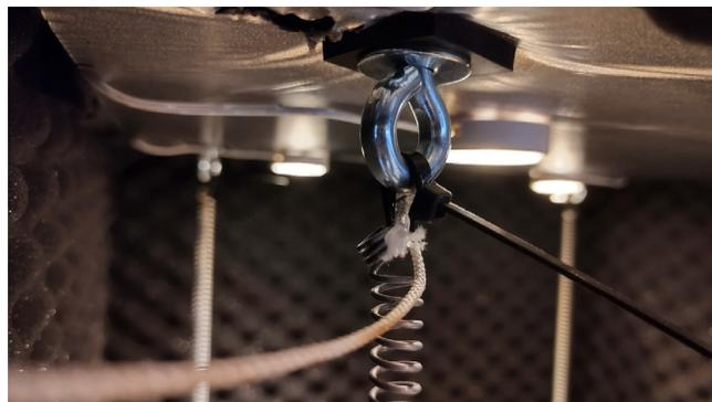
Fig. 27. Springs connected to eyebolts with zip ties.
