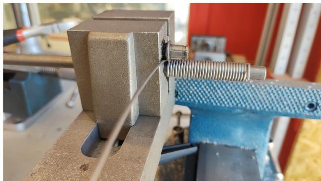
Fig. 25. Spring steel winded in spring winding tool.
