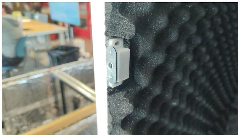
**Fig. 13.** Cut away foam to fasten the magnet.
