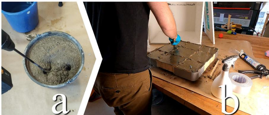
**Fig. 23.** a) Mix concrete thoroughly in accordance with package. b) Pour concrete, distribute and pack it with a stick.
