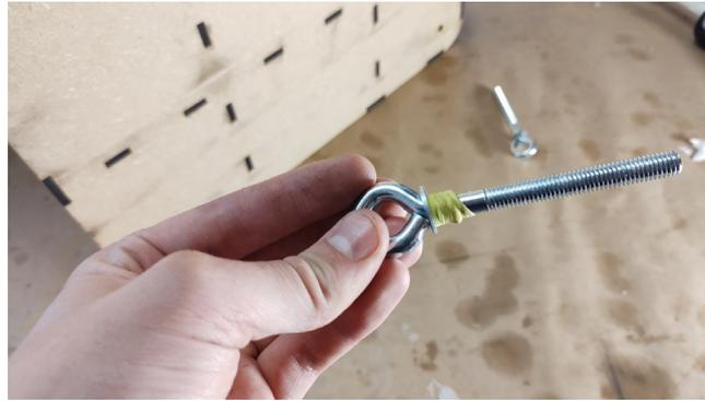
**Fig. 21.** Gasket made of vacuum bagging sealing tape.
