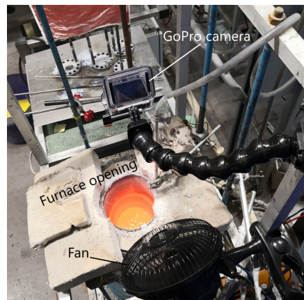
Figure 3. Image of the experimental setup with the camera placed above the surface opening.
