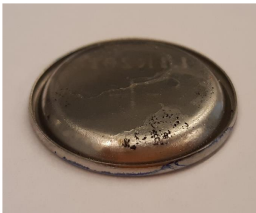
Figure S6 Signs of side reactions on the bottom steel casing after performing the 200 h hold step at 1 mV vs. Mg/Mg 2+ with the APC-THF electrolyte, after being rinsed in THF.
