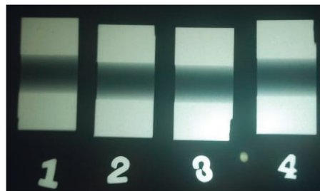
FIGURE 5: X-ray radiography of the printed components.
