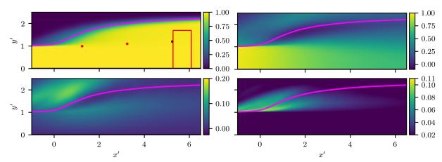
**Figure 3.** Distribution of  $\langle \alpha \rangle$  (top left),  $\langle u \rangle / U_1$  (top right),  $\langle v \rangle / U_1$  (bottom left), and  $\langle k \rangle / U_1^2$  (bottom right) in the benchmark simulation. The magenta line shows  $\langle \alpha_{0.5} \rangle$ .
