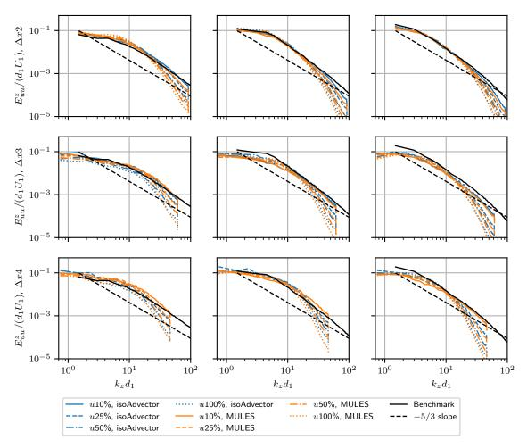
**Figure 14.** The spanwise velocity spectra obtained in the simulations at three selected locations: [1.24, 1] (left); [3.24, 1.1] (middle); [5.24, 1.4] (right).
