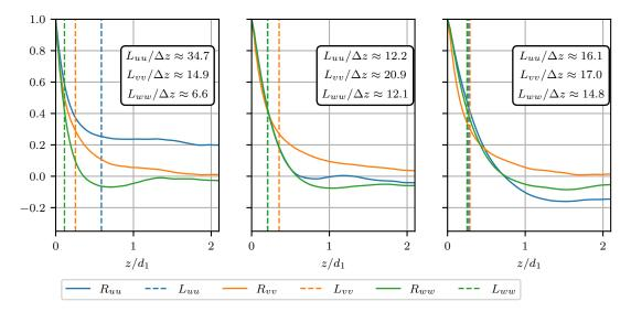
**Figure 9.** Spanwise two-point auto-correlations of velocity components computed at 3 selected [x', y'] locations: [1.24, 1] (**left**); [3.24, 1.1] (**middle**); [5.24, 1] (**right**). Vertical dashed lines show the integral length scales.
