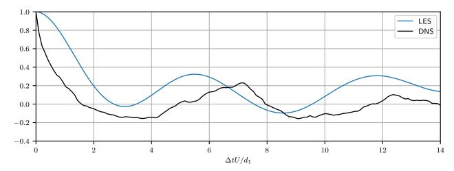
**Figure 10.** Autocorrelation function of the time signal of the air volume passing through the box  $x' \in [5.27, 6.09], y' \in [0, 1.70].$
