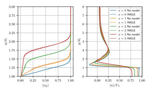
**Figure A1.** Effect of explicit SGS modelling using the WALE model. Profiles of the volume fraction of air (**left**) and streamwise velocity (**right**).
