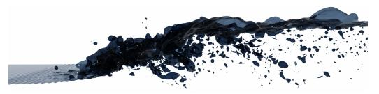
**Figure 1.** Classical hydraulic jump at  $Fr_1 = 2$ ; a snapshot of the air–water interface.
