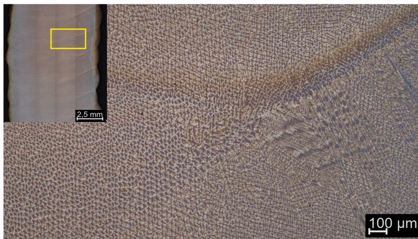
(b) Flower intersection. Mixture of columnar and equiaxed dendrites.
