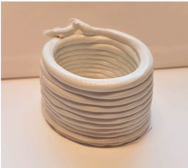
Fig. 2. Cylindrical cup-structure built in preliminary experiments described in Preliminary tests with viscous material. Approx. 4 cm tall, built using a viscous glue.
