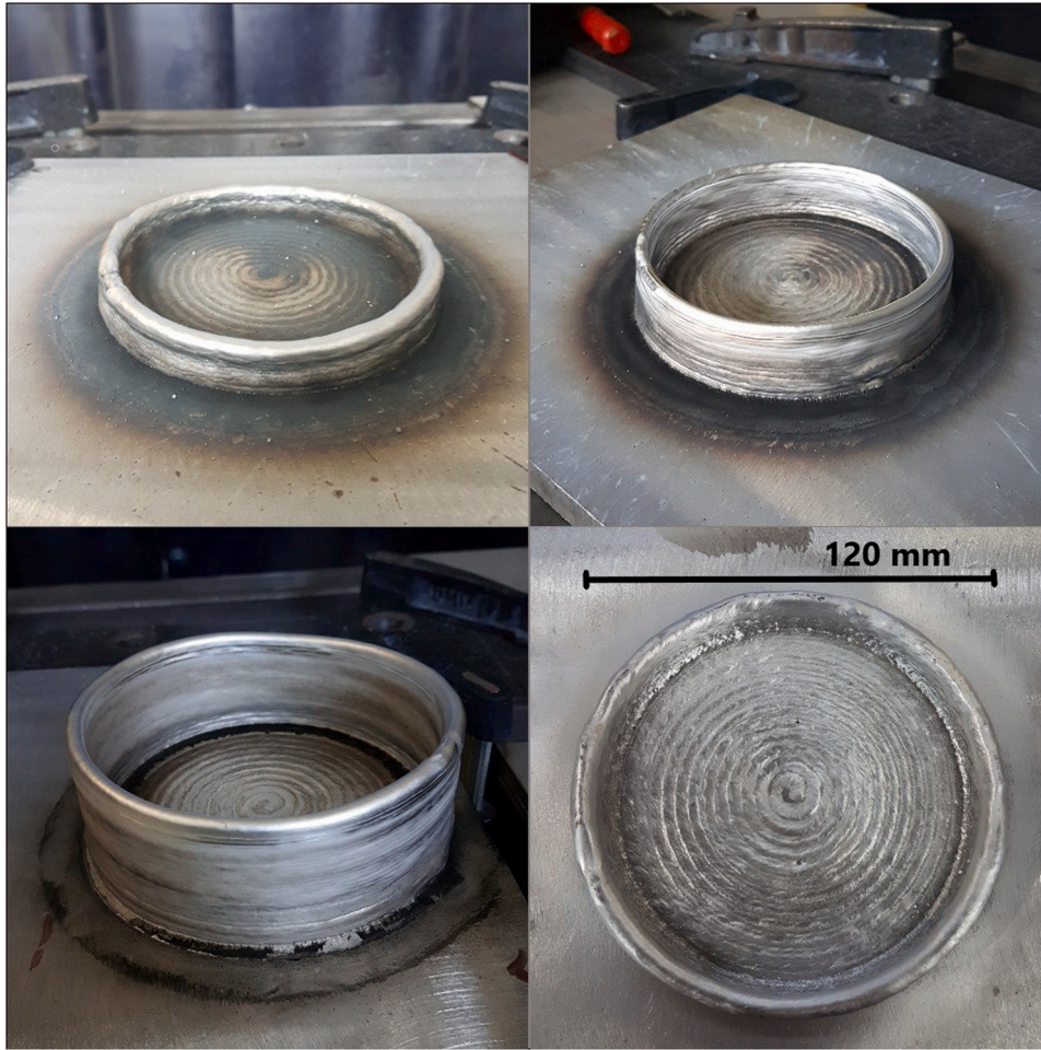
Fig. 8. Set-based: The structure was a cylindrical shape. The bottom layer was constructed in a outwards spiral, while the path for the wall was an upwards helix with a constant radius and a constant height increase.
