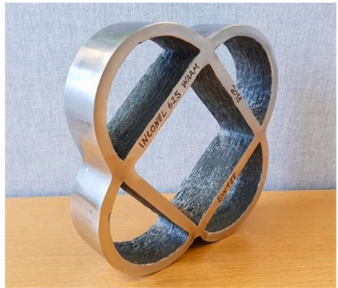
(b) Second, modified CMT box build with smoother walls and few distortions.
