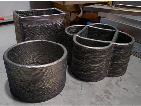
Fig. 19. Additional structures were constructed in the Ni-Cr-Mo alloy UTP 759.
