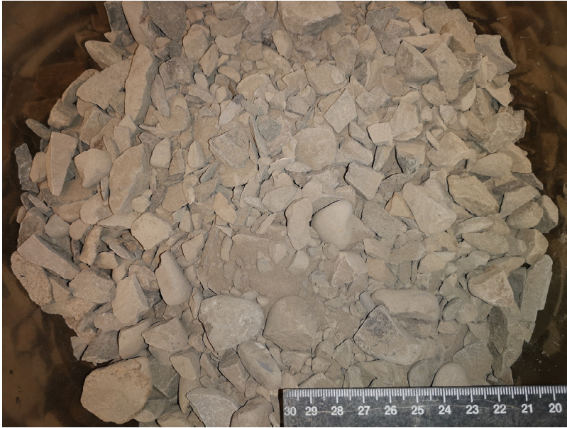
Fig. 11. Loose material tested with RLTTs.
