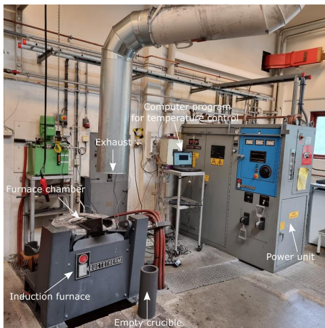
Figure 3.3: A photograph of the 75kW induction furnace and the crucible used in this work
