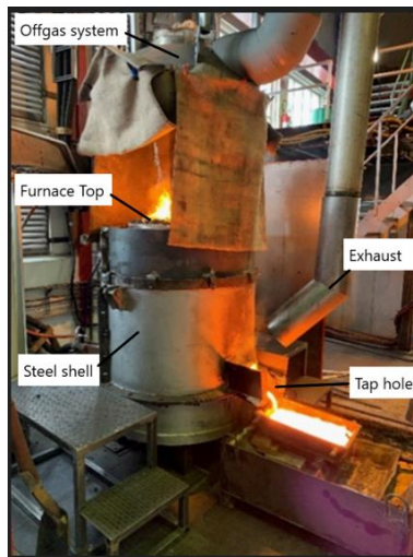
Figure 4.3: A photograph of the pilot furnace in operation
