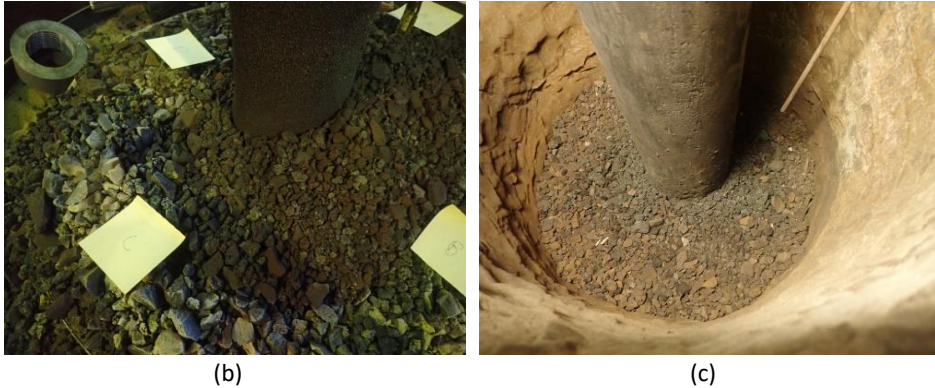
Figure 4.23: (a) A schematic illustration of the sampling regions during the furnace digout and a plan view of the SINTEF/NTNU Pilot furnace. (b) Photographs of furnace top prior to dig-out & (c) interior of the furnace and top of cokebed after complete digout of the prereduction zone.
