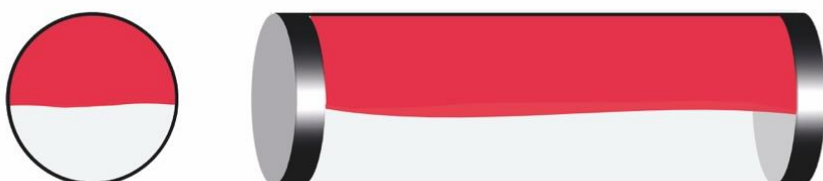
Figure A5. Stratified flow of water and oil. [O & W].
