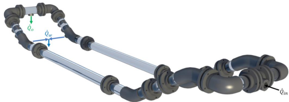
Figure 6. Prototype of parallel pipe bulk oil–water separator.
