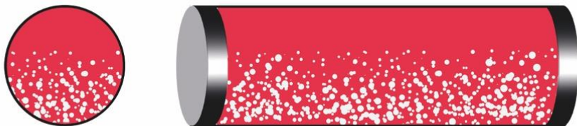
Figure A3. Oil and dispersion of water in oil. [O & Dw/o].
