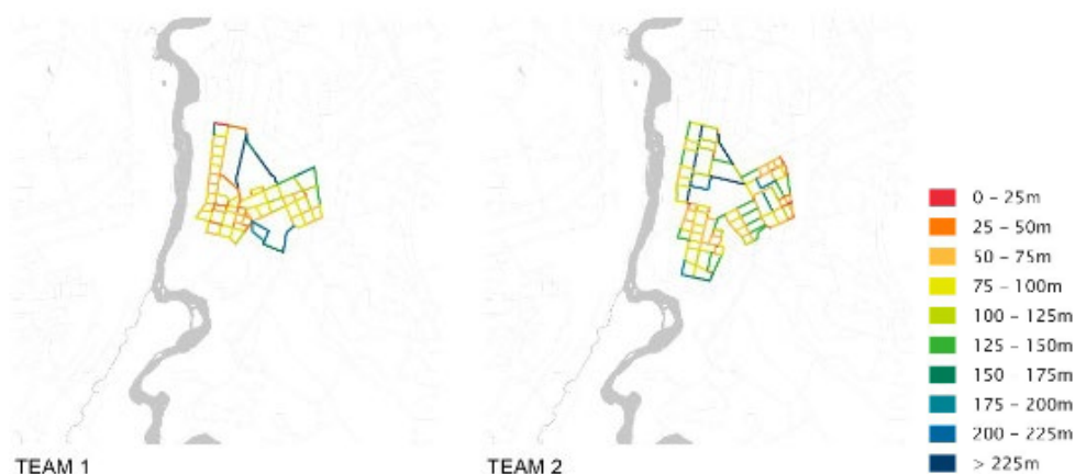
Figure 36. Calculated street intersection density for two plan proposals within the ZEN pilot area Sluppen (55).
