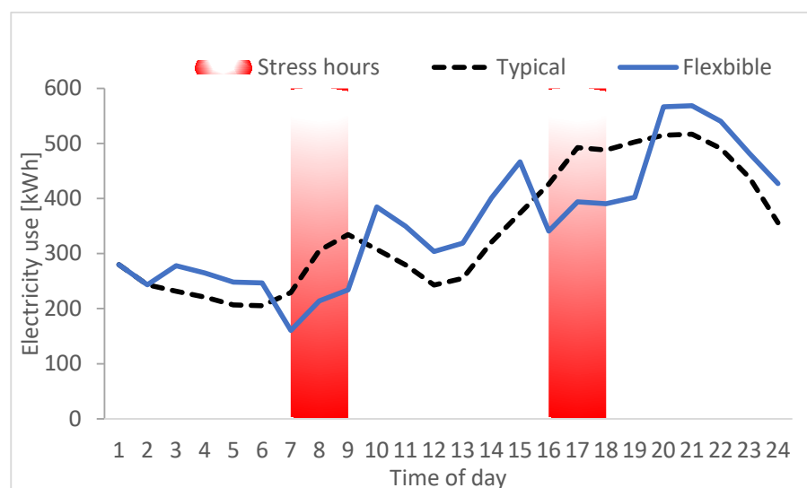
Figure 25 Alternative load profiles in a neighbourhood with (flexible) and without optimal control (typical) to reduce energy in the stress hours.
